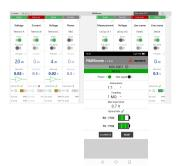
The system is delivered with montena FibREmote software for PC and Android devices. The application allows simple configuration and monitoring of the optical link(s).
