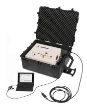
This portable generator is used to verify the performance of protective devices at the electrical point-of-entry of fixed ground-based facilities or transportable systems against high-altitude electromagnetic pulse (HEMP) according to MIL-STD-188-125 (PCI: pulse current injection).
