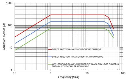
Examples of direct current injections in a 50 ohm load
