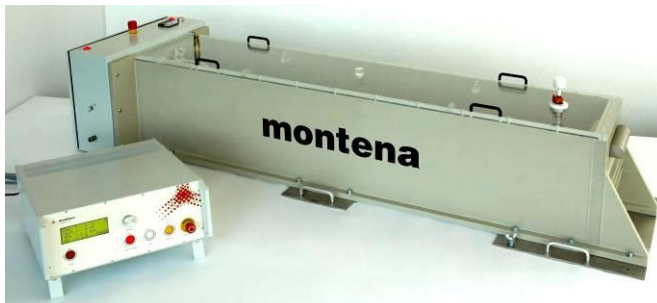
Fig. 3: Marx + peaking 360 kV NEMP pulse generator
