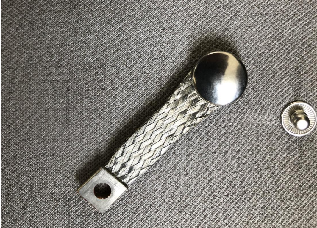
Picture 3: using textile rivets to establish electrical contact to the ground plane
