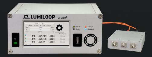
The LSPM 1.1 / LSPM 2.1 Laser-Powered RF Power Meters can also be combined with the Computer Interface CI-250+. It is equipped with a 4.3" Touchscreen and Ethernet Interface.
