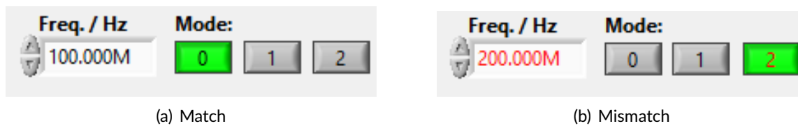
Figure 21: Frequency control for matching (a) and mismatching (b) TCP server and GUI settings
