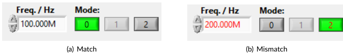
Figure 24: Frequency control for matching (a) and mismatching (b) TCP server and GUI settings
