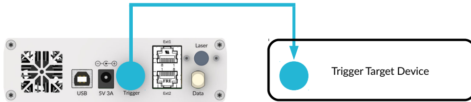
Figure 12: External trigger output using BNC connector
