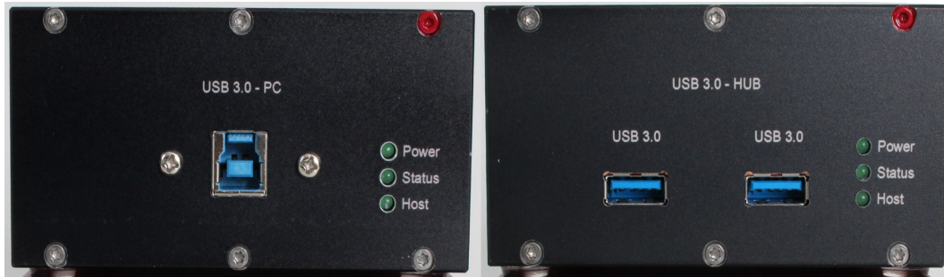
Fig. 7.2: Rear side of the devices – PC side on the left, HUB side on the right
