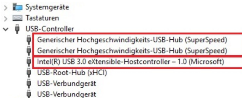
Fig. 1: Drivers for USB3.0 host controller has to be installed by the operating system of the PC
