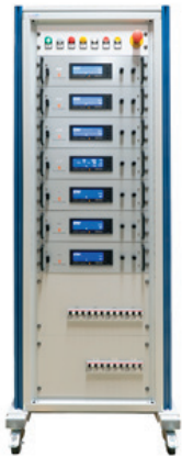
LV 123 System, 105 kW
