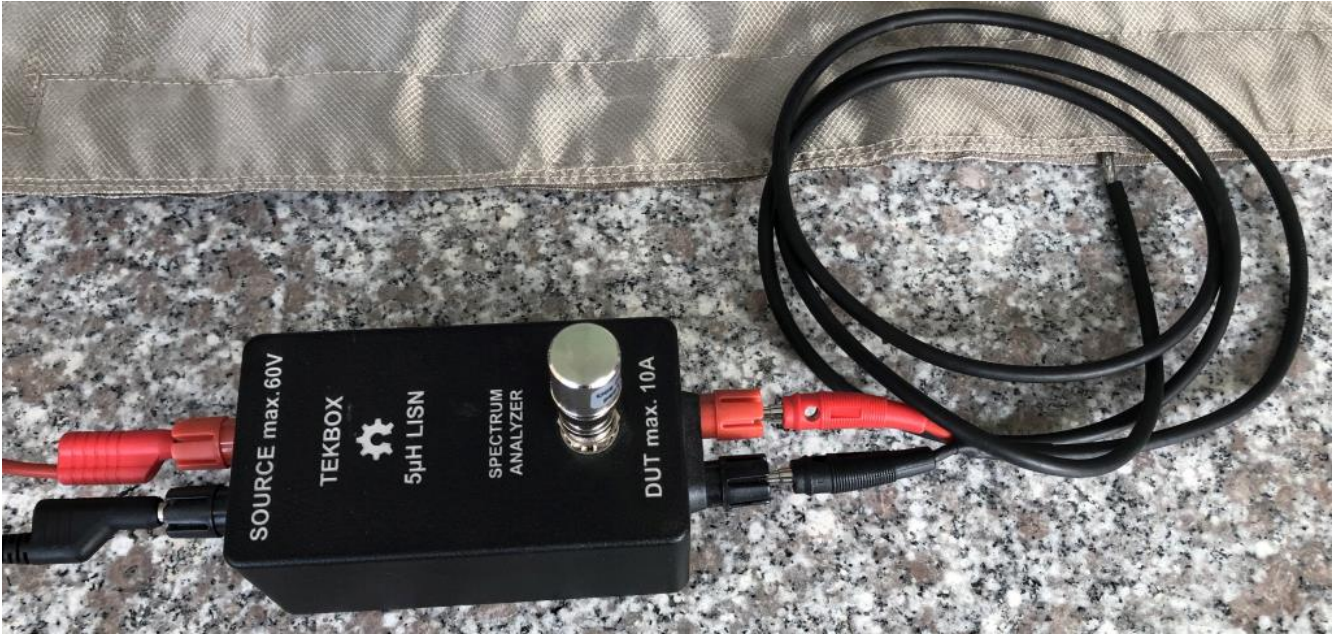
Picture 17: DUT supply feed through using a shielded cable and a 5µH LISN as supply line filter
