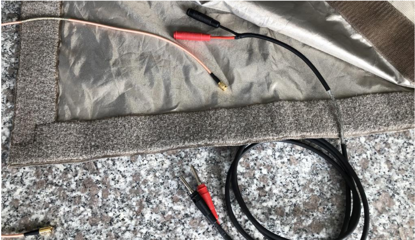
Picture 14: DUT supply feed through using a shielded cable with stripped jacket
