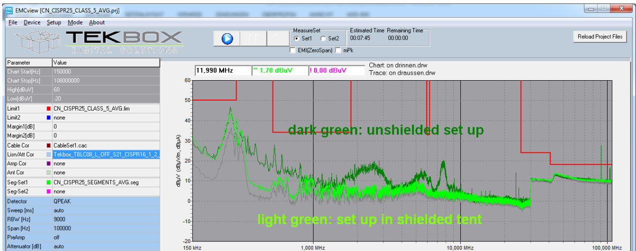
Picture 6: CISPR 25 conducted noise measurement; DUT powered
