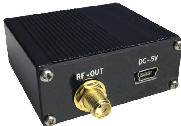
Picture 2 – TBWA2 wideband amplifiers rear view
