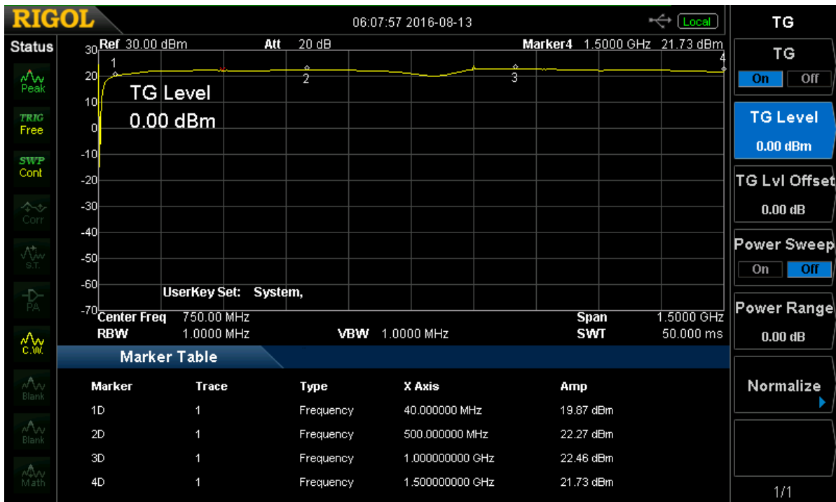
Picture 8 – output power of the TBMDA1, CW, driven by the DSA815 tracking generator set to -1dBm
