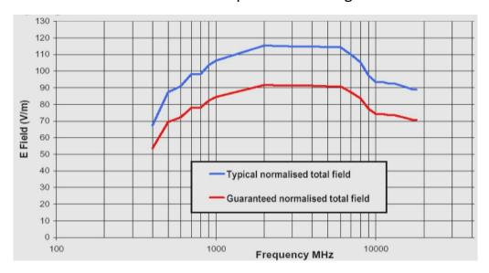
Normalization field with 1W radiated power according to the IEC-61000-4-21 and MIL-STD 461F Standard.
