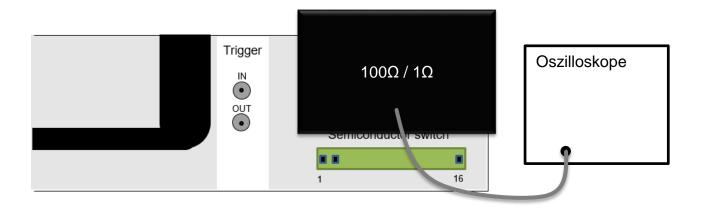
The CAR-PFS-R-CAL Kit avoids, with its short connections, additional inductances. If you use another resistor, the reference resistor shall be connected as close to the "+OUT" and "-OUT" sockets of the CAR-PFS as possible.
