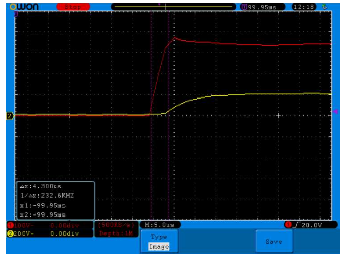
Figure 44 Fall time and rise time @ 90 degrees in the order of 3 – 4 \mu S, for the 1 cycle starting @ 90 deg
