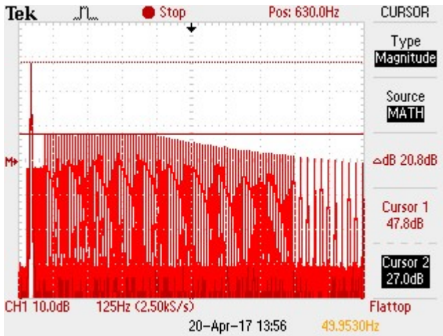
Figure 51 The Meister Curve sweep test 16.5 – 2000 Hz
