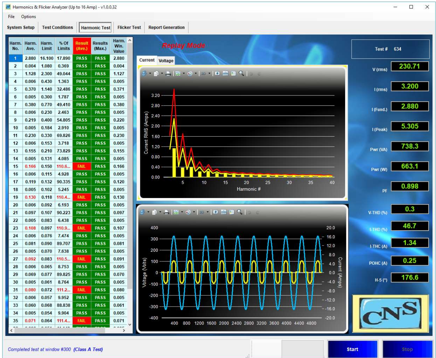
Figure 9 Test screen of a Class-A test with several harmonics exceeding the 100 % limits.
