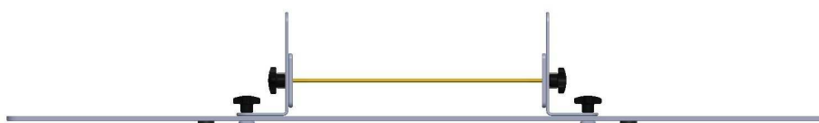
Abb. 3: Line 1 Kalibrierstandard (für hohe Frequenzen) Fig. 3: Line 1 calibration standard (for high frequencies)
