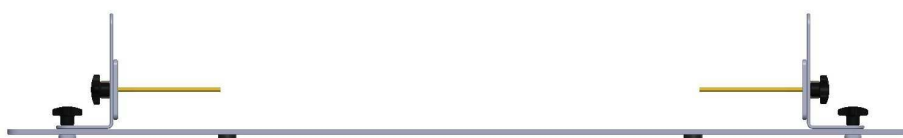
Abb. 1: Reflect Port 1 und Reflect Port 2 Kalibrierstandards Fig. 1: Reflect Port 1 and Reflect Port 2 calibration standards
