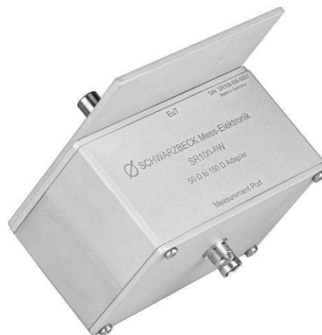
Abb. 2 Serienwiderstand SR-100-6W Series resistor SR-100-6W
