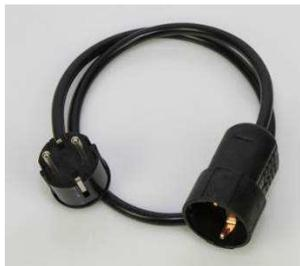
2x 0.8 m 3-pole cable, CEE7/4 jack (connector to EuT) to CEE7/4 plug (to CU CEE7/4, AMN), EN 50561-1, chap. 6.2, fig. 2
