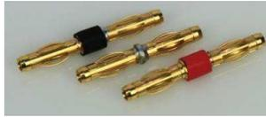
*Spare: 2x connectors (red and black) consisting of two 4 mm laboratory plugs each, connected back to back, ~38 mm length, 1x connector (blank) consisting of two 4 mm jacks connected back to back, ~32 mm length*
