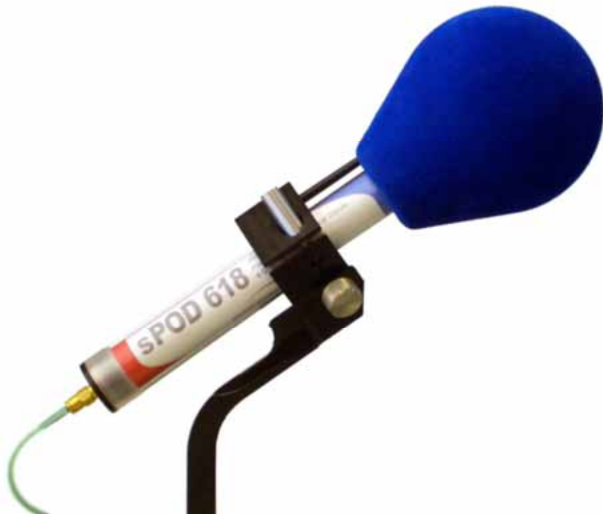
Figure 19: sPod mounted on a Field Nose rotator for Add3D measurements
