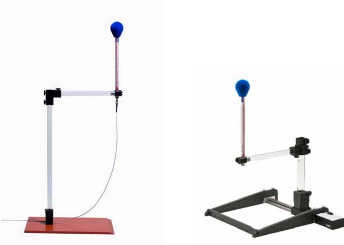
Figure 4: Site VSWR Positioner Left: SPM1: Manual Positioner with POD Antenna mounted in vertical polarization Right: SPA1: Automatic Positioner
