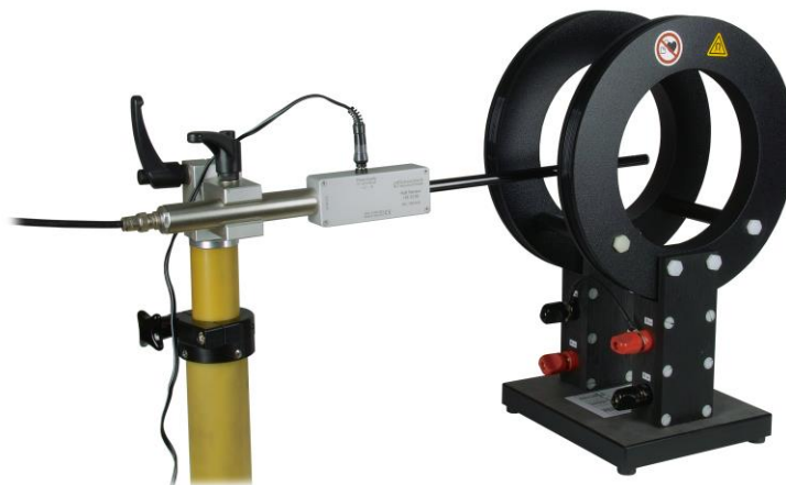
Abb. 4: Messaufbau Hall-Sensor in Helmholtz Spule Fig. 4: Measurement setup Hall sensor in Helmholtz coil
