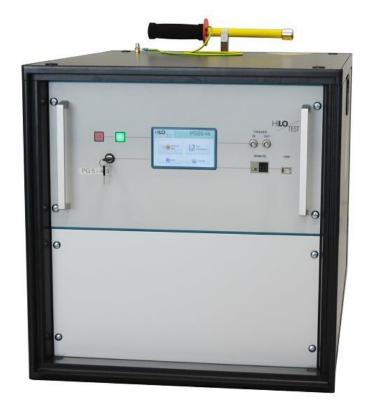
The high-voltage impulse generator PG 20-4000 generates standard impulse voltages with waveform 10/700 µs. Output voltage is adjustable between 1 kV and 20 kV. The polarity of the output voltage is selectable, positive or negative.
