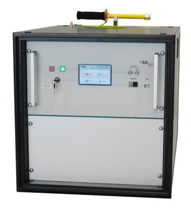
The high-voltage impulse generator PG 14-1960 generates standard impulse voltages with waveforms 10/700 µs. The output waveform can be switched to 0.5/700µs wave. Output voltage is adjustable between 0.2 kV and 14 kV. The polarity of the output voltage is selectable. Positive, negative or alternating polarity of the output voltage can be preselected.
