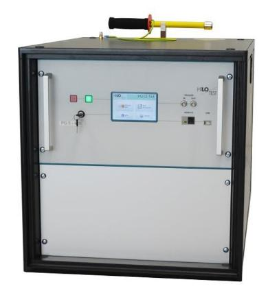
The high-voltage impulse generator PG 12-1440 standard impulse voltages with waveforms  $1.2/50~\mu s$  or  $10/700~\mu s$ . Output voltage is adjustable between 0.5 kV and 12 kV. The polarity of the output voltage is selectable. Positive, negative or alternating polarity of the output voltage can be preselected.
