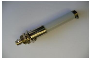
The Broad-band pulse voltage divider, type PVD is a state-of-the-art measuring equipment whose excellent high-frequency transmission characteristics can be fully exploited only if properly operated and if all aspects typically encountered in the sub-microsecond time region, e.g. appropriate grounding, transmission line characteristics of leads, are fully considered.
