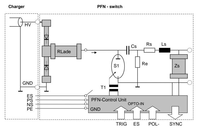
The energy storage capacitor C is charged via the charging resistor. The diodes D1 and D2 are used to protect against reverse polarity of the charger. By triggering the switch S1 of the energy storage capacitor Cs is discharged via the discharge resistor Re and the series impedance Rs + Ls. The desired HV pulse is generated.
