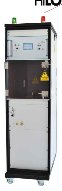
The surge current generators PG20-14000 generate standard impulse currents with waveform 8/20 µs according to IEC, EN, VDE. Pulse current output amplitude is controlled by preset charging voltage and can be adjusted up to 100 kA.
