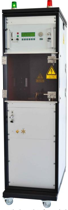
The pulse-forming network contains a pulse-fidelity current viewing resistor for monitoring the output waveform. The impulse current output is located at the top of the equipment and provides high-current bolts M12 with a changing test adapter M12.
