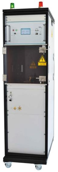
The surge current generators PG20-7000 generates standard impulse currents with waveform 8/20 µs according to IEC, EN, VDE. Pulse current output amplitude is controlled by preset charging voltage and can be adjusted up to 50 kA.
