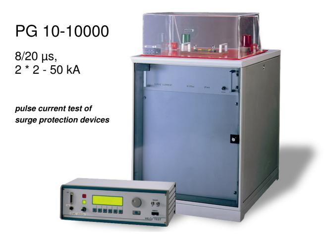
The SURGE TEST GENERATOR PG 10-10000 delivers surge current pulses with the waveform 8/20µs, acc. to IEC 60. It was designed for testing surge protection devices. Moreover the generator can be used for testing two-gap over-voltage protectors. It delivers surge current pulses synchronous at two impulse current outputs, peak value adjustable 0.5 - 50 kA for each output. Positive or negative polarity of output current can be selected.
