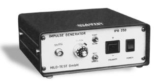
The pulse generator IPG 250 is designed for measuring the step response of high-impedance networks, for instance voltage dividers, oscilloscope probes etc. The generator excels by calibrated adjustment of output amplitude, short rise time and flat pulse top. The output pulse amplitude can be adjusted by use of a 10-turn potentiometer from 0 to 250 V. Positive and negative polarity can be selected.
