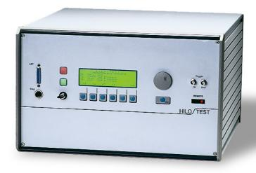
HV - Impulse generator PG 4-641 creates standard voltage and current pulses with wave form 10 / 160  $\mu$ s. Output voltage is adjustable up to 3600 V, the maximum short circuit current amplitude is 480 A peak. Positive or negative polarity of output voltage can be selected. A built-in voltage divider 1000:1 allows monitoring of the impulse output waveform during testing. The short circuit current wave can be monitored by use of the built-in shunt.
