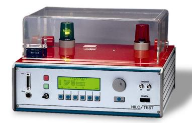
The High-Voltage Pulse Generator Type IPG 809 is designed for dielectric testing of X- and Y-capacitors with standard impulse voltages  $1.7/46 \ \mu s - 0/+50\%$  up to 8 kV acc. to IEC 60384-14, EN 132400, VDE 0565 etc.
