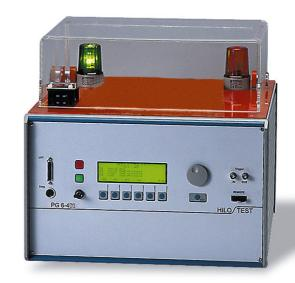
The High-Voltage Pulse Generator Type PG 6-401 is designed for dielectric testing of X- and Y-capacitors with standard impulse voltages  $1.6/47~\mu s$  up to 6 kV acc. to IEC 384-14, etc. The generator has the same principle of operation as the IPG 809 but allows testing capacitance values of 33 nF - 470 nF.
