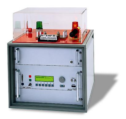
The high-current pulse generator PG 6-2402 is designed for surge current testing of electrical components, over-voltage protectors and electronic circuits acc. to IEC, VDE etc. It generates standard impulse currents with waveform 8/20µs. Pulse current output amplitude can be set to 2 - 50 kA.
