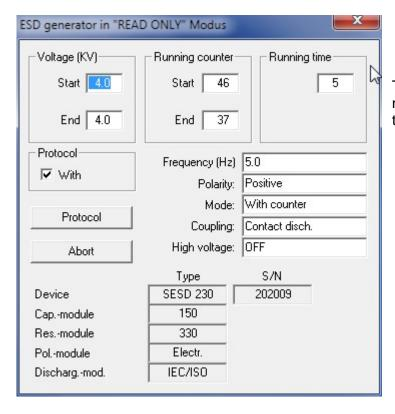
The function READ ONLY allows a notification of the manual operation with the ESD generator.
