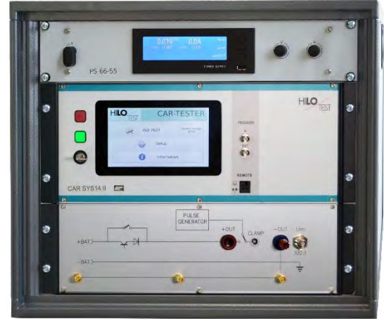
Figure 12: CAR TEST SYSTEM with option PS 66-55 to extend by Pulse 2b and Pulse 4.
