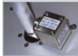
OPT. VT 20 dB plug in divider to measure high field strength
