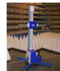
High Load Antenna Mast
