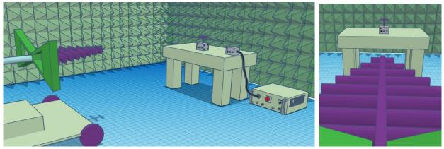
For use in conducted immunity, the comb generator is connected directly into the EUT power port of the LISN or Telecom ISN. The injected signal can then be measured with the receiver to verify the measurement path.
